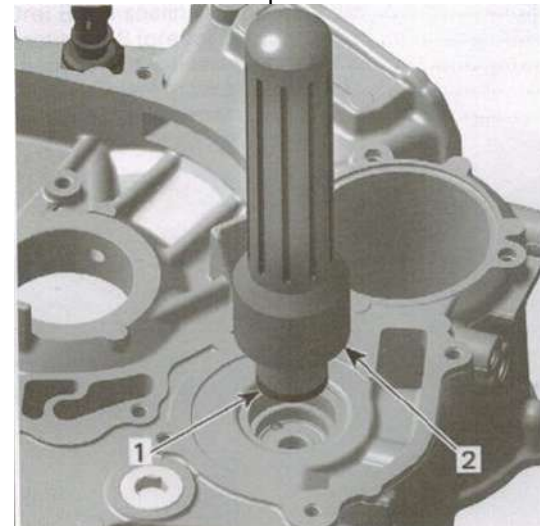
1.Inner oil seal 2.Installer handle with oil seal pusher
