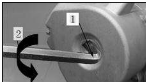
1. Allen key 14mm 2. Turn crankshaft 280° counterclockwise
