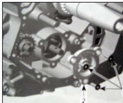
1. Retaining screws 2. Oil pump cover
