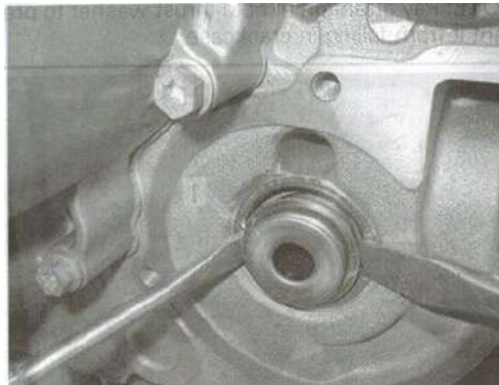
To remove outer part of rotary seal, use an expander from puller kit.
