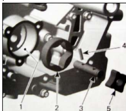
1. Oil pump bore 2. Outer rotor 3. Oil pump shaft 4. Needle pin 5. Inner rotor
