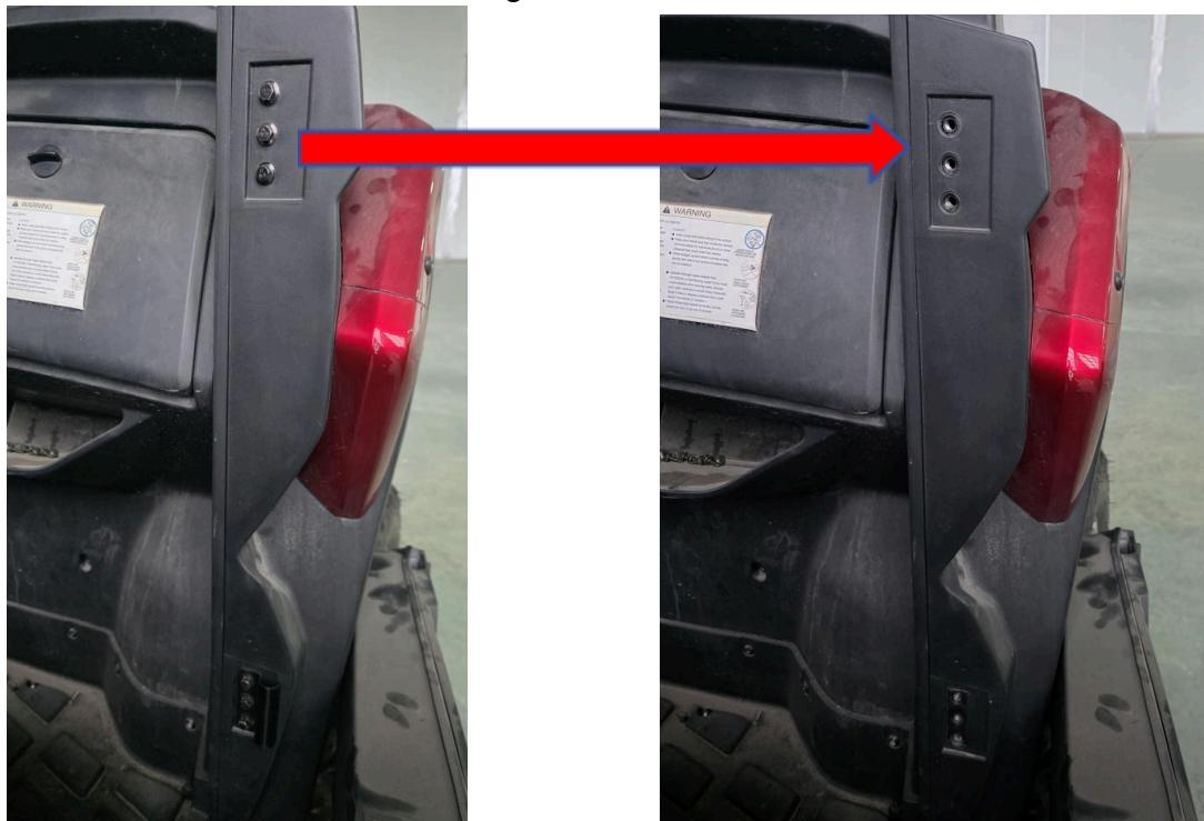
4. Finally, fit the half-door hinge to the vehicle with six M8×25 countersunk hexagon socket bolts as shown in the diagram.
