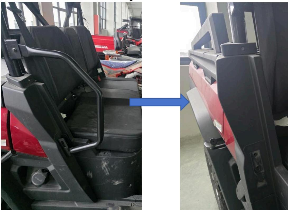
2. Fit the side door striker with two M8×25 hexagon socket cap head screws at the side armrest removal position, as shown in the diagram.
