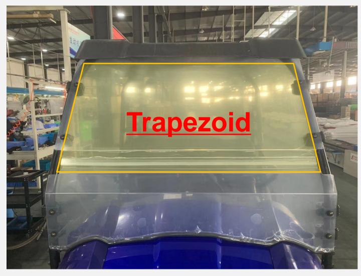
The upper section of the windshield installation position frame is trapezoidal.
