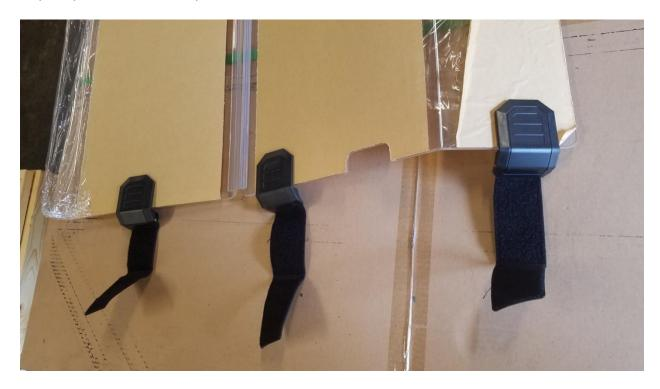
Step 4 Position the windshield against the front bars. A second set of hands will help to hold it in place. Place a piece of cardboard on the vehicle hood to protect the surface until the windshield is installed and in place.
