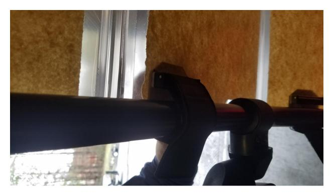
It is easiest to start with the middle clamp on each side. Then, move the windshield up or down to get the proper position and proceed to the other clamps. Finally, pull the Velcro straps tight to secure the windshield in place. The brown paper can then be peeled off the windshield.
