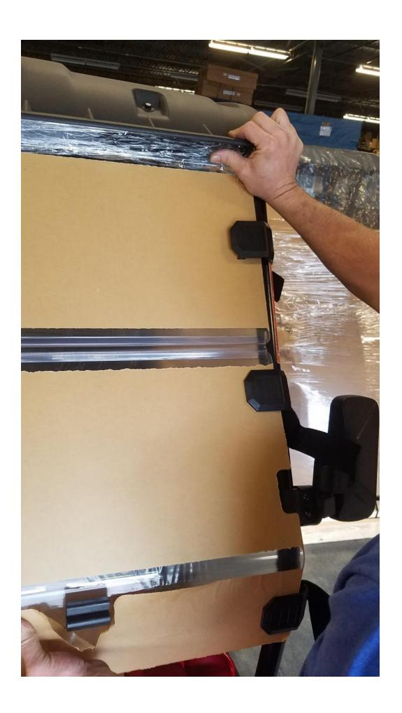
Step 5 wrap the Velcro strap around the bar, slide the strap under the metal bar, and then fold it back on itself to close the Velcro. Align the mirror brackets with the cutouts in the windshield and secure the mirrors I place. This will assure the proper positioning of the windshield and prevent it from moving.
