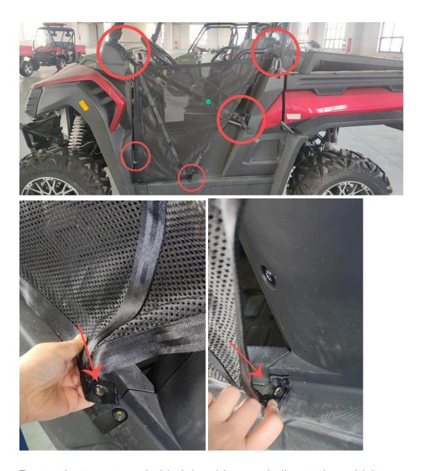
Fasten the two straps behind the side guardrail onto the vehicle.
