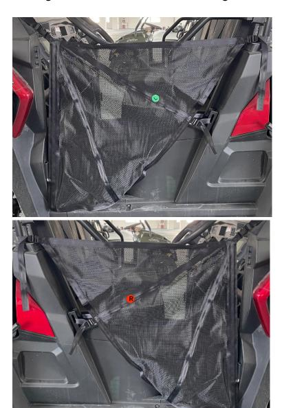
First, determine the installation position of the side guard. Then loosen the specific bolts on the vehicle. Place the corresponding parts of the side guard in the designated position, and then tighten the bolts to secure the side guard.
