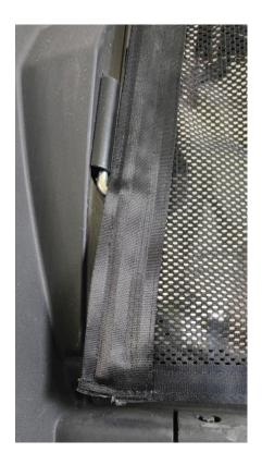
Fasten the buckle in front of the side guard to the vehicle. The installation order on both sides should be consistent.
