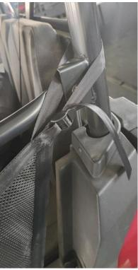
Insert the pins in front of the side guardrail into the installation plate on the vehicle.
